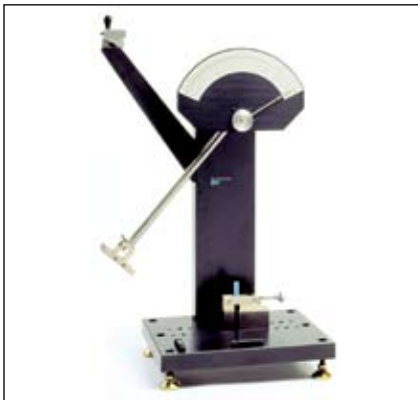
Charpy Impact Test Configuration
