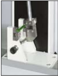
Charpy Impact Test Configuration
